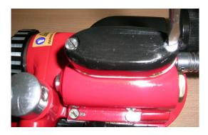
When the bearing cover is dropped of, the nut of the right bearing (112.084) must be detached.
