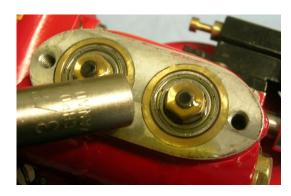
Following resolve the three screws (112.053) on the body and unplug the complete motor inclusive the turbine shaft (115.092) out of the pistol.
